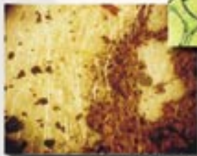
Filtered rust particles
